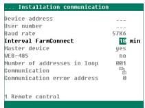
Sample setting on external device: FarmConnect interval = 10 minutes by default
