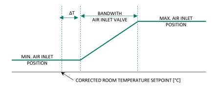
To set the minimum and maximum air inlet positions and the bandwidth, press several buttons in succession.
