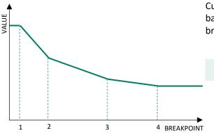
Curves allow you to pre-program the climate process based on the age of the animals. To set a curve (max. 4 breakpoints), several keys must be pressed in succession.
