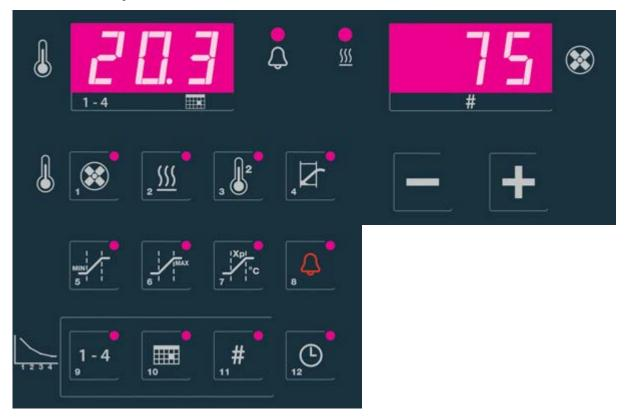
When no lamps are lighting up on the operation panel, the temperature measured in the room is shown on the left display and the current ventilation of the room on the right display.
