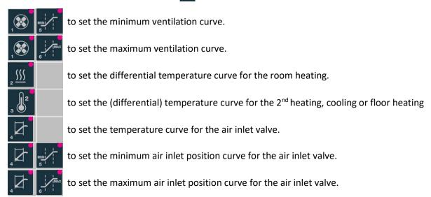
For example, use key combination , and 1-4 to set the day number of the minimum ventilation curve.
