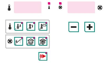
When no lamps are lighting up on the operation panel, the current boiler water temperature is shown on the left display and the current ventilation of the central exhaust on the right display.
