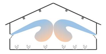
For floor housing, the AeroWing SC can be installed at a low For aviary or cage housing systems, the AeroWing SC can be additional advantage of this is that obstacles at roof height, such as roof trusses, lighting or winch-suspended feed and water lines, do not affect the air distribution.
