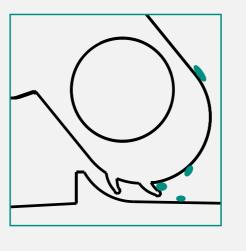
The air inlet uses the venturi effect to draw in the air inside the house along with the incoming air. The round opening keeps the air in the house moving to prevent condensate from forming on the valve.
