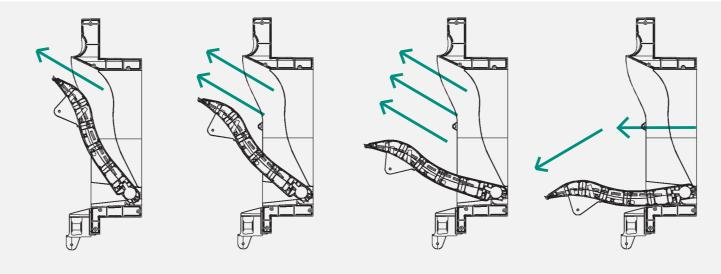
Lowering pressure drop: If the ventilation level is 70% or higher, the pressure can be lowered to apply displacement ventilation.
