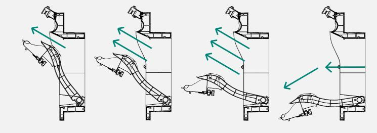
Lowering pressure drop: If the ventilation level is 70% or higher, the pressure can be lowered to apply displacement ventilation.
