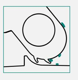
The air inlet uses the venturi effect to draw in the air inside the house along with the incoming air. The round opening keeps the air in the house moving to prevent condensate from forming on the valve.
