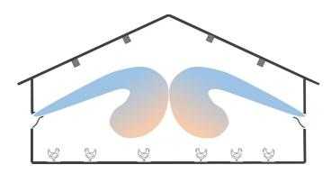
For floor housing, the AeroWing can be installed at a low height, since the air throw is independent of the roof slope. An additional advantage of this is that obstacles at roof height, such as roof trusses, lighting or winch-suspended feed and water lines, do not affect the air distribution.
