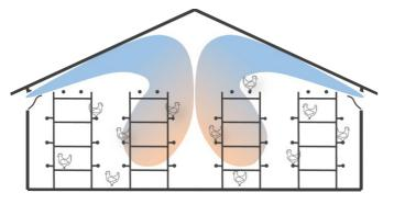
For aviary or cage housing systems, the AeroWing can be placed high up to ensure ventilation between the roof and the
